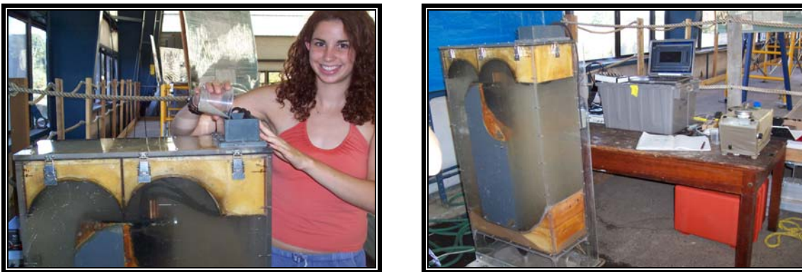
Figure 1: Jennifer Miller adding 1g/L to racetrack (left). Experiment set up, including: racetrack, personal computer with DAQ card, and weighing scale (right).
