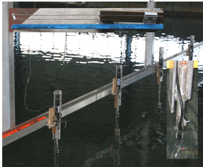
Figure 2. Instrument array on I-beam.
