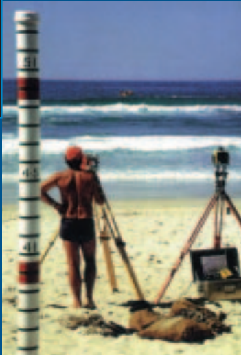
A beach profile being surveyed as part of the COPE field experiment at Burleigh, Gold Coast.
